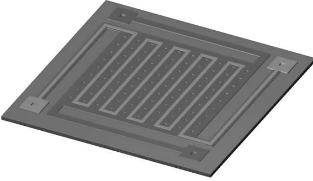
Figure 5.14 Bolometer formed in Poly2 layer of a PolyMUMPS process. A serpentine resistor forms a suspended temperature sensor that is thermally isolated from the substrate.
