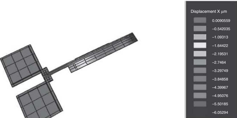
Figure 5.9 Displacement of the heatuator. The tip of the heatuator deflects by more than 6 \mu\text{m} . (Reprinted with permission from IntelliSuite v8.6 (2010).) See color plate section.
