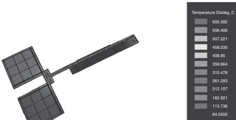
Figure 5.8 Temperature distribution for the heatuator. The hot arm heats up to more than 600°C. (Reprinted with permission from IntelliSuite v8.6 (2010).) See color plate section.
