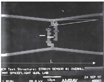
Figure 2.16 Bent-beam strain sensor for characterization of residual stress. Under tensile stress the arms will deflect outward. Under compressive stress the arms will deflect inward. (Reprinted with permission from J. Microelectromechanical Systems, Bent-beam strain sensors , Y. B. Gianchandani and K. Najafi, ©1967 IEEE.)
